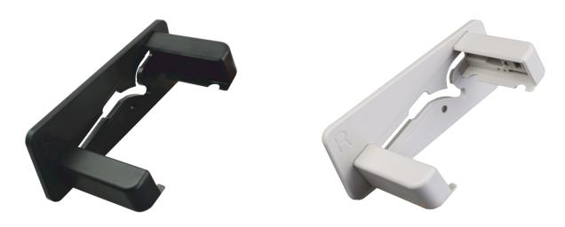
The Bracket Holder Mounting Kit is a construction set to fix Elatec's TWN readers on a flat surface. Available in white and black color, it consists of one ground plate and two brackets with screws and a double sided strong adhesive pad. It can be assembled for left or for right side mounting. For optional additional screwing, an extra hole located on the base plate.
