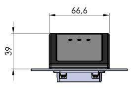
\*All drawing measurements in mm
